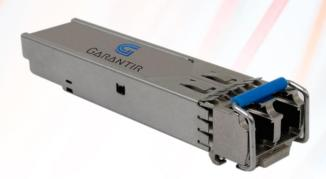
Garantir Small Form Factor Pluggable 10G SFP+ transceiver are high performance, cost effective modules supporting upto 10Gbps / 10G Ethernet speed. They are RoHS compliant and lead-free. Transceivers are compatible with SFP (Small Form Pluggable) Multi-Source Agreement (MSA). These transceivers having high density LC connector interface and are Hot-swappable.
