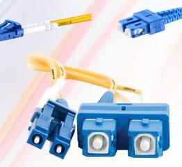
Fiber Patch cords are basically jumper cables for the connection of fiber optic equipment to equipment or LIU panel to equipment. It comprised of a patch cable terminated with connectors. There are many variations for fibers, cables and connectors. For fiber, it can be Singlemode or Multimode (50um, 62.5um, OM3 etc.) type. As for cable, there are simplex and duplex types. For connector, to name a few common ones are SC, & FC.
